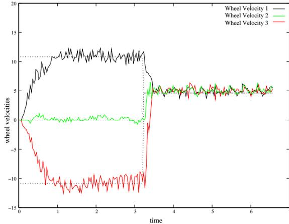
Fig. 4. An exemplary trajectory of the robot using the learned motor controllers. The solid lines show the achieved velocities of the three wheels while the dashed lines show the desired wheel velocities.
