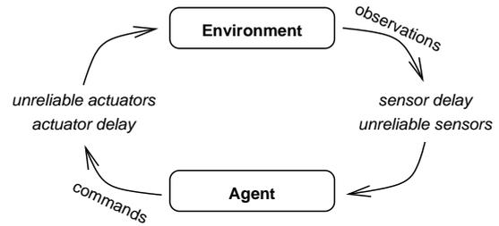
Fig. 1. Adaptation of the classical world-agent interaction loop to the situation with which we are typically faced with in autonomous robotics
