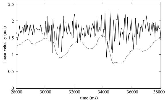
Fig. 3. Comparison of three velocity measures: desired linear velocity (dashed line), odometry (solid line) and estimated linear velocity (dotted line). The robot was given motor commands with constant linear velocity and varying angular velocity.
