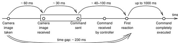
Fig. 2. Illustration of the time gap due to sensor and actuator delays.
